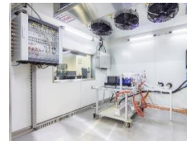
Fuel cell system test stand 160 kW with climate chamber
